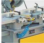
Adjustable Horizontal Pneumatic Clamping
